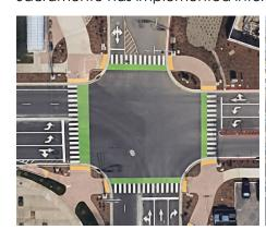
**Protected Intersections** physically separate bicycles from motor vehicles through the intersection providing people biking with a ages and abilities. Bicycle signal heads may also be provided.
