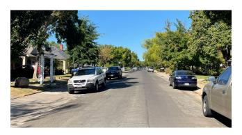
On Street Parking: Reduces roadway width by allowing parking along a roadway curb, causing a driver to experience increased "friction" on the side of the road resulting in lower driver speeds.
