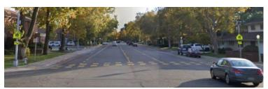
**Rectangular Rapid-Flashing Beacons** are user-actuated yellow flashing lights to improve safety at uncontrolled, marked crosswalks. They are used to alters drivers to yield where people walking have the right-ofway crossing a road.
