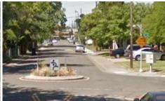
Roundabouts/Traffic Circles are a type of intersection where traffic is permitted to flow in one direction around a center island. Traffic approaching the roundabout yields to traffic already within the intersection.
