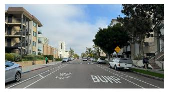
Lane Narrowing: Narrowing lanes to 11 feet reducing the total of space vehicles have. This provides a visual cue for drivers to slow down through painted striping or adding a bikeway.
