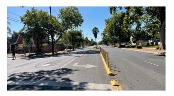
Hardened Centerline: Treatments are typically a flexible delineator post of raised speed hump along the road centerline at an intersection to narrow the path through the intersection, slowing turning drivers.
