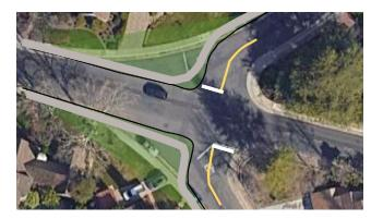
**Curb Radii / Geometry Changes:** Changing roadway geometry or narrowing curb radii increases the amount of curb space, requiring vehicles to slow down when turning. This treatment can also be used to realign skewed intersections to right angles.
