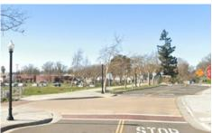
Curb Extensions, also known as bulb-outs or neckdowns, extend the sidewalk or curb line out into the travel or parking lane, which reduces the effective street width.
